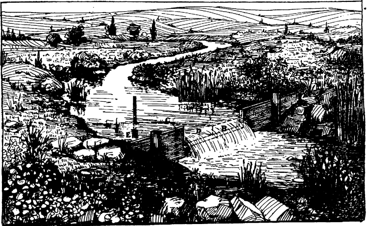
FIG. 11.—The weir method of stream measurement. A board is set across the stream, with a notch cut deep enough to pass all the water. Measurements are taken at a stake, E, and from these the quantity of water can be determined by means of a table given in the text.
